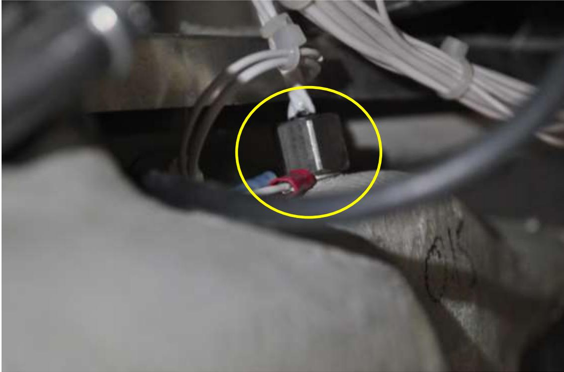
Figure 1: Grounding wire attached to the OAT probe
